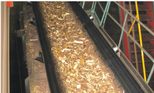
Minnesota Power's Rapids Energy Center woody biomass feed.
